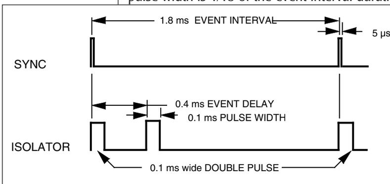
Vary the three PULSE GENERATOR dials and notice how the waveform timing follows the dial values. Note that the OUTPUT light is dimly lit, reflecting the fact that the pulse width is 1/18 of the event interval duration. Try to extend the pulse into the next event interval. This may be accomplished by increasing the delay or increasing the pulse width or decreasing the event interval. As soon as the pulse width overlaps the beginning of the next interval, the VIOLATION light should illuminate.
